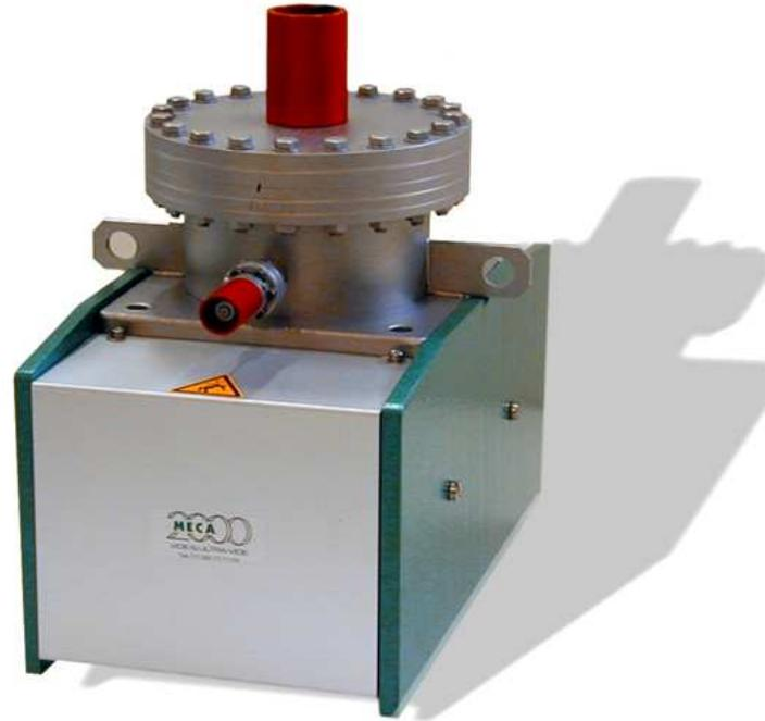
Meca 2000 ion pumps have diode pump elements and meet all requirements of UHV applications in terms of pumping speed, stability and lifetime.. They can reach pressures down to  $10^{-12}$  mbar due to their UHV design. They require no maintenance and are easily started from  $10^{-4}$  mbar. They are often used in installations permanently kept under vacuum.
