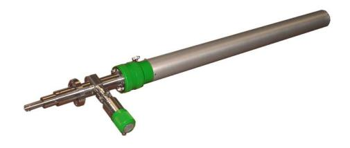
All mechanical transfer rods in the CTLT series are reliable and very precise products, allowing users to work in UHV technology at pressures down to 10<sup>-12</sup> mbar. These transfer rods provide a combined movement of rotation and translation around and along their axis, with the advantage of installation in all positions. These movements may be motorized and controlled by a joystick upon request. The CTLT series rods are available on CF40 or CF63 flange.
