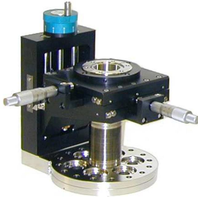
The manipulation instruments for linear motion have been designed to ensure the movements of components and samples under Vacuum and UHV ( $10^{-12}$  mbar) with great precision.
