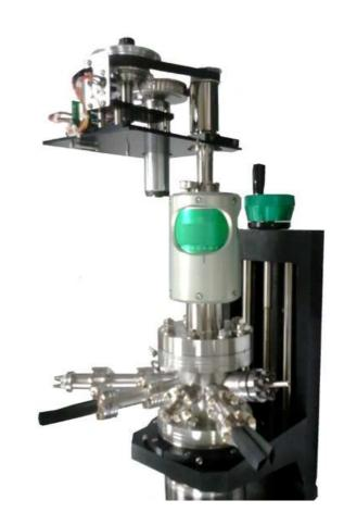
The manipulation instruments for rotary motions have been designed to ensure the movements of components and samples under vacuum and UHV (10<sup>-12</sup> mbar) with great precision.
