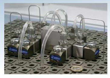
The modular concept allows the build-up of several different plant configurations, reactor lengths and sampling points depending on the selected reaction process. For example, a reaction section can be build up with two A3 plates in series in order to get a total reactor available length of 9 m (with 4 x 4 mm<sup>2</sup> channel cross section) consisting of six horizontal 'meander reactors' (three reactors by plate) in series.
