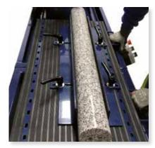
SLABBING UNIT SLABBING UNIT SLABBING UNIT
