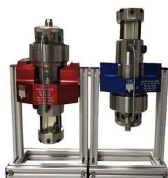
Six H2-brine centrifuge coreholders (imbibition & drainage)
